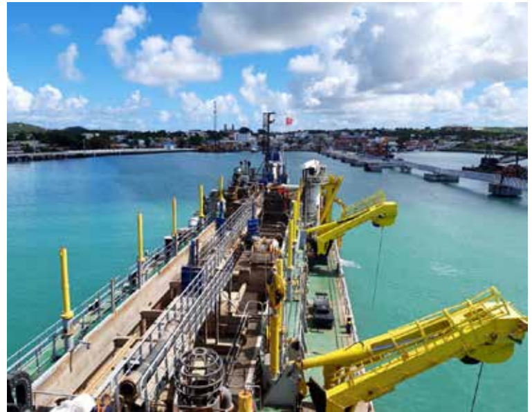
The trailing suction hopper dredger, Elbe, is one of the pieces of equipment that was used by Blue Ocean Marine Ltd. to conduct dredging work at the St. John's Harbour.
